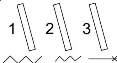
Sharpening a badly blunt or damaged blade.
